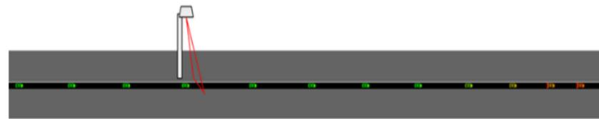
FIGURE 2 : A graphic representing the road geometry combined with a single radar sensor generating aggregate speed measurements.
