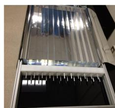
Fig i: Scintillator bars
