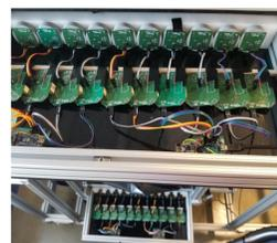
Fig ii: The PCBs and SiPMs
