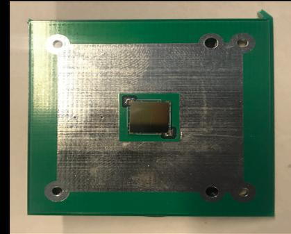
Fig 3. Silicon Photo Multiplier (SiPM)
