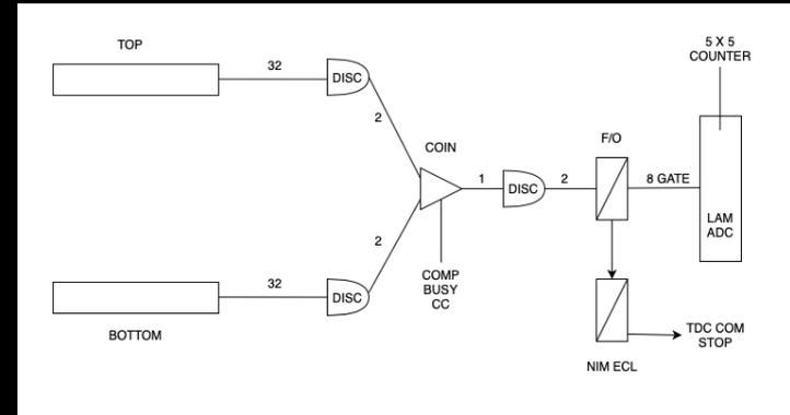
Fig 2. DAQ Trigger Process.
