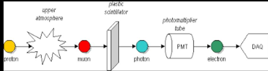
Fig 1. Schematic summarizing the muon detection process
