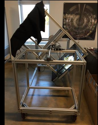
Fig 4. Muon Telescope
