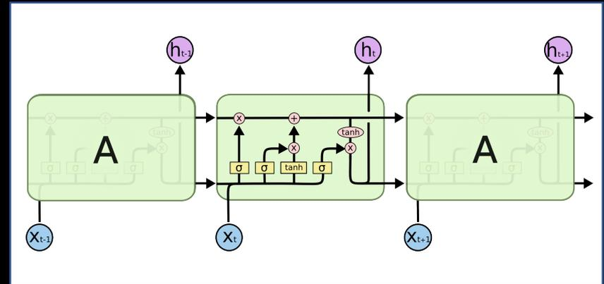
Fig 1. LSTM Cell Structure
